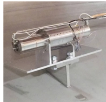
Liquid Argon pump allows if needed to pump LAr out of the cryostat for a liquid phase purification cycle
